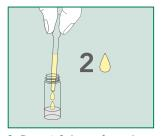
2. Deposit 2 drops of sample into the diluent bottle.
